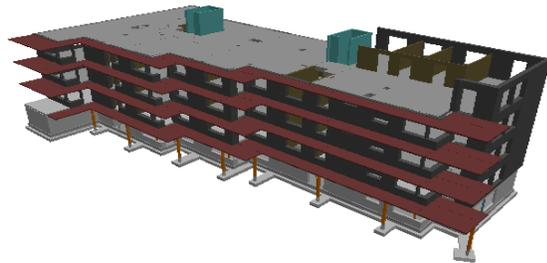
Stage 2. Some of the wall elements on the fifth story are being installed.
