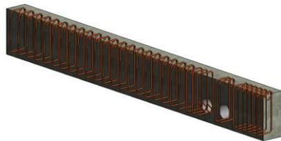
Finally, at LOD 400, highlighted in table 9, the element is modeled with exact geometry showing the finishing chamfers and all reinforcement detailing ( $G_3$ ). Failure modes are also checked and various situations are considered such as construction sequence and the location of construction joints ( $C_8$ ).
