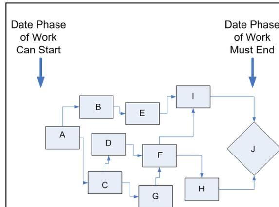
Figure 9: Logic Network-after buffer is distributed
