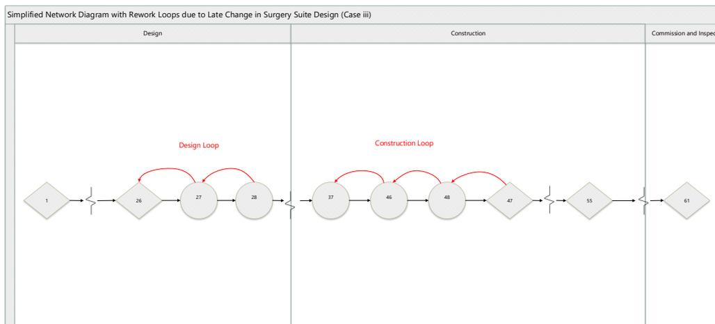
Figure 12: Proactive strategy Case iii - Simplified network diagram with rework loops due to arrival of new information for dental clinic design
