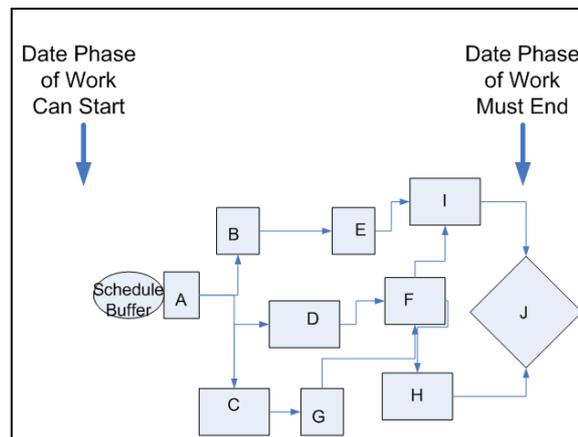
Figure 8: Logic network-with schedule buffer
