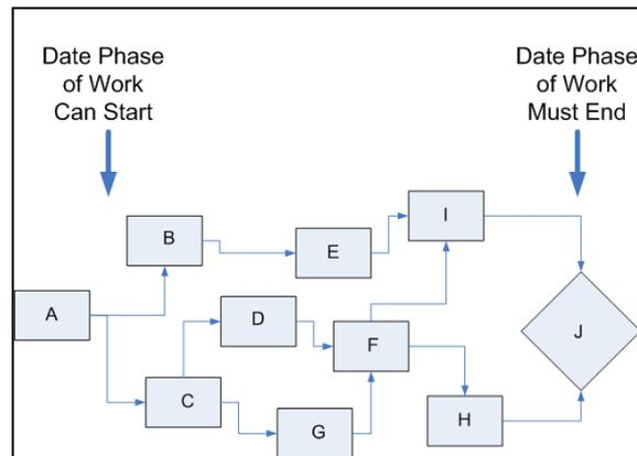
Figure 7: Logic network-does not fit within available time
