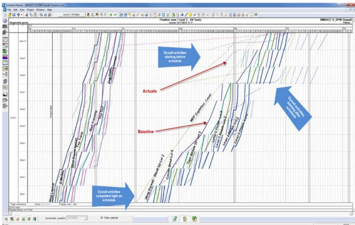
Figure 5. Line-of-Balance Analysis (courtesy DPR, Inc.)
