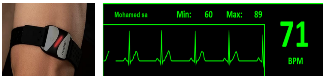
Figure 5. The pulse rate sensor and its location on the participant's arm on the left; the captured pulse rate data via the Cardia application in real-time on the right.
